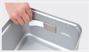
When you placed indicator band inside the box, you should be sure that placed references and indicator should appears. You should specify the suitable position by reciprocating motions or rotating reverse the indicator band.
